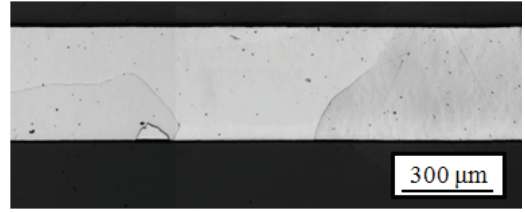
Fig. 2 Optical micrographs of the annealed samples at 950°C for 10 min in hydrogen atmosphere
