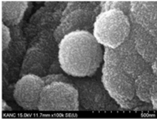
그림 1 FESEM of ZnS:Ni nanospheres showing that nanospheres are consisted of much smaller nanoparticles.
