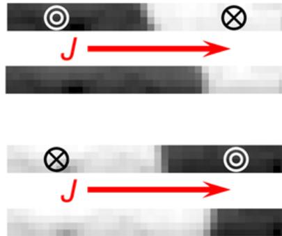
Fig. 1. DW motion along the current flow observed in Pt/Co/Pt device with symmetric Pt thicknesses. Black(white) domain represents up(down) magnetic domain, respectively.
