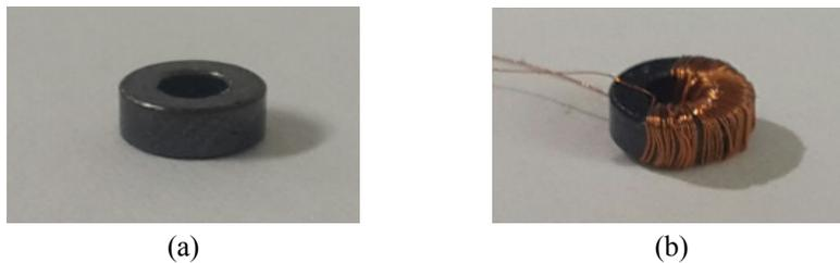
Fig 1. Photographs of ferritecore(a) and toroid sample(b)
