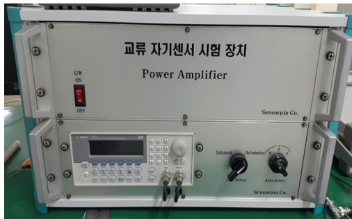
Fig. 3. Frequency bandwidth measurement of the magnetometer.
