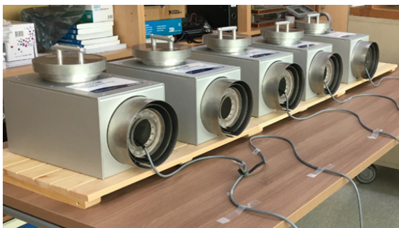
Fig. 4. Long term drift measurement of the magnetometer.
