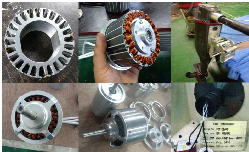
Fig. 1. Prototype of BLDC motor for Electric Outboard Propulsion
