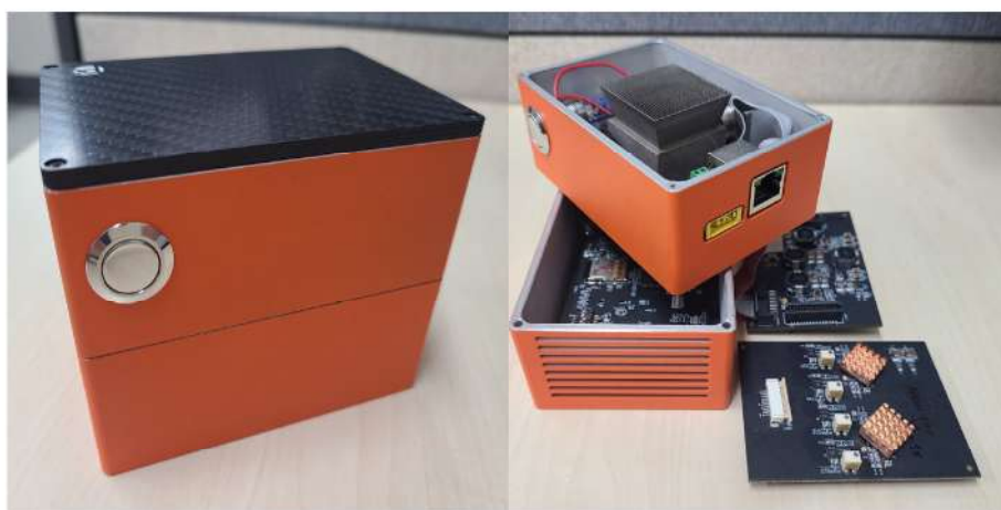
Fig. 1. Appearance of the compact gamma camera and proposed SoC-FPGA and SiPM
