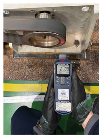
Fig. 14. (Color online) Experimental setup. (a) Test Configuration, (b) Coupled Configuration of the Test Motor and Generator, (c) Speed Measurement.
